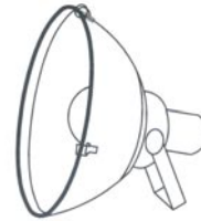
Type A floodlight giving a symmetrical beam
